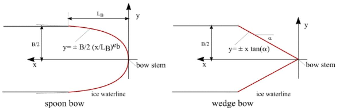
Figure 8 - Illustration of  $e_b$  Effect on the Bow Shape for  $B = 20$  and  $L_B = 16$
