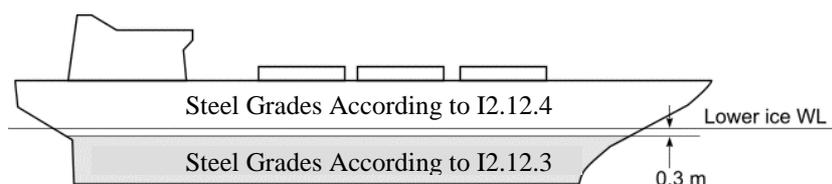
I2.12.4 Steel grades for all weather exposed plating of hull structures and appendages situated above the level of 0.3 m below the lower ice waterline, as shown in Figure 6, are to be not less than given in Table 6.
